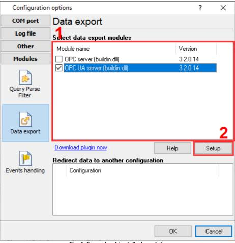
Fig. 1. Example of installed module
